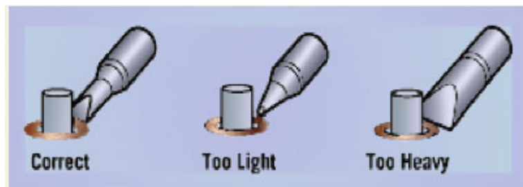
Figure 11: The tip should have a similar width to the object being soldered
