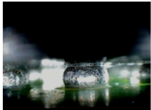
Difference in Ball shape, surface finish, and stand off height between lead free and traditional tin/lead alloys
