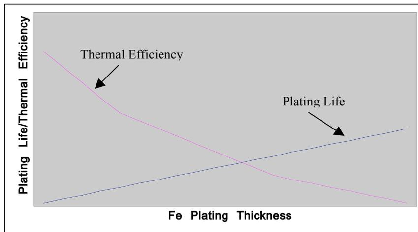
Good quality plating and good tip care techniques will have a significant improvement on plating life and heat transfer efficiency
