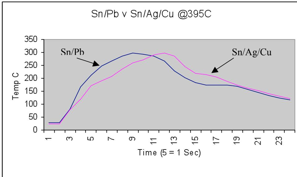
The second set of profiles compare the two different soldering temperatures. It can be seen that at lower tip temperatures the solder flow/joint formation phase is longer. The maximum joint temperature reached is also lower, although the temperature difference appears to be quite small. Interestingly the rate of temperature rise during flux activation is greater at the lower tip temperature and the overall soldering time similar.
