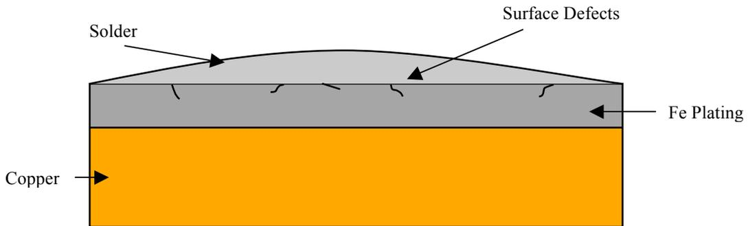
The molten solder starts to penetrate into these surface defects. This is called the defect initiation phase and represents the largest portion of the time to failure
