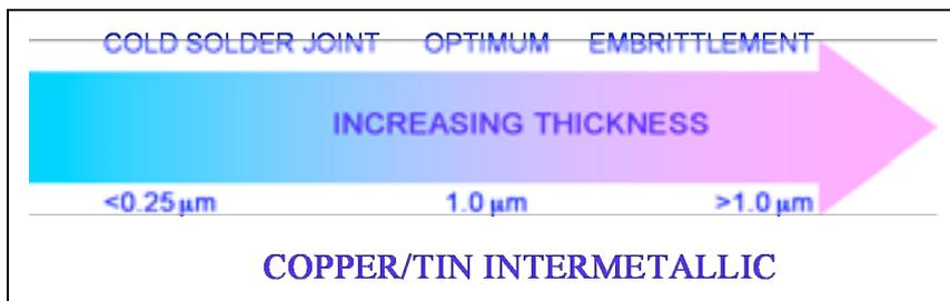
Intermetallic layer thickness can be an indication of joint quality
