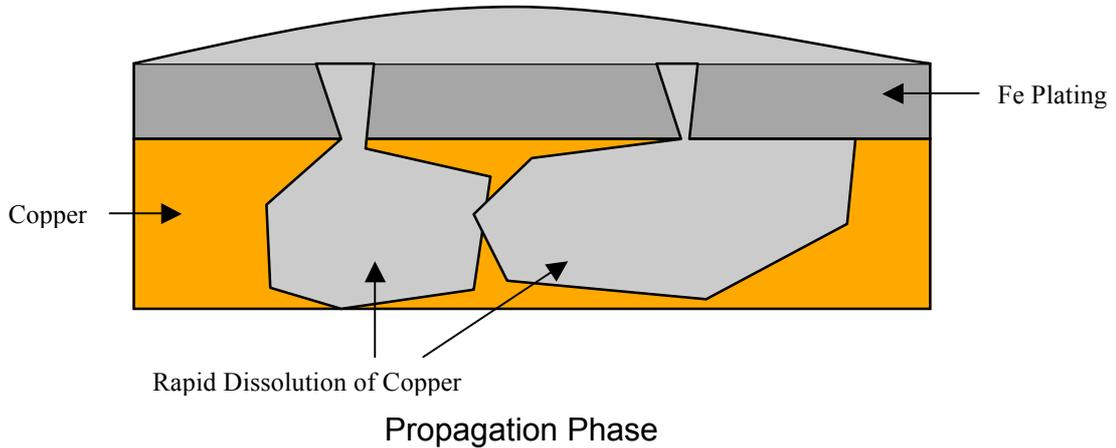
Increasing the thickness of the iron (Fe) plating will increase the life of the tip however iron (Fe) has a relatively poor thermal conductivity and so the overall thermal transfer efficiency of the tip will be significantly reduced.
