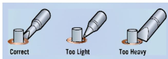
The tip should have a similar width to the object being soldered
